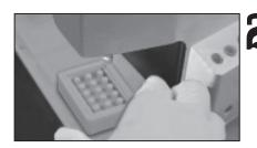
Slowly dispense liquid paraffin (60 °C to 65 °C) until the top of core rods are fully submerged. If bubbles are formed, remove them with a pair of heated forceps. For recommended paraffin, most histologists prefer using Paraplast X-Tra®. Others use Formula "R"<sup>TM</sup> Paraffin or Blue Ribbon<sup>TM</sup> from Leica Biosystems. These sticky paraffins will help cores adhere better then harder ones in the recipient block.
