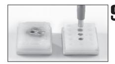
By slowly pushing on the T-Sue<sup>™</sup> punch needle plunger, deliver the extracted tissue into the corresponding hole of the recipient block. Then, gently push in all the tissue cores to ensure evenness for microtomy.
