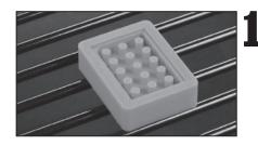
Place the T-Sue<sup>™</sup> Array mold in an oven for 30 minutes at 70 °C to 80 °C.
