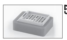
Cool at room temperature or at about 4 °C for 30 to 60 minutes. Warning: At lower temperatures, cracks may appear in the block.
