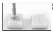
Extract the marked tissue from the donor block by using the appropriate T-Sue<sup>™</sup> punch needle.
