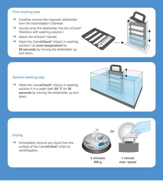
Figure 6: Working steps of the washing and drying procedure prior to the analysis of the CarnoCheck<sup>®</sup> chip with the CheckScanner™ and the CheckReport™Software.
