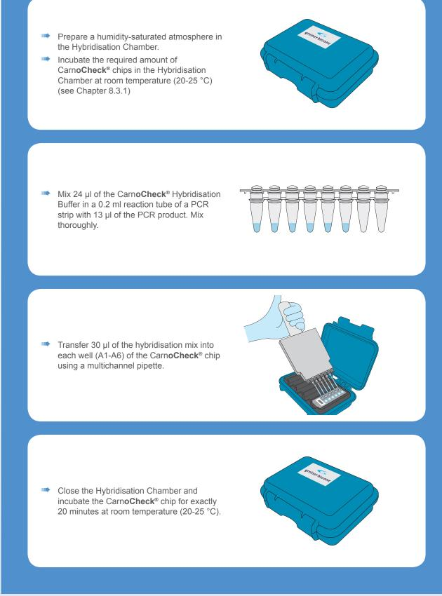
Figure 5: Working steps of the hybridisation procedure
