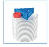
5 The CELLevator™ must be positioned within the circumferential ring of the top plate of the CELLdisc™.
