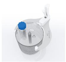
CELLhandle facilitates secure and easy transportation of particularly largesized CELLdisc™ formats as well as convenient emptying of these.
