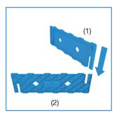
**1** Join segment (1) with segment (2) using the indentations. Centering ribs at the side of the indentation guide the segments together.
