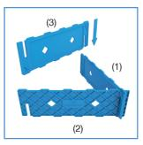
**2** Join segment (3) accordingly with the indentation of segment (1) from above.
