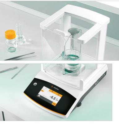
**Increase Efficiency with Integrated Application Programs** Quintix<sup>®</sup> comes standard with convenient, built-in applications. These, along with the extensive accessories Sartorius offers, enable you to customize Quintix® to a variety of weight measurement tasks. Take specific gravity. With the built-in Density application and the Sartorius Density Kit, you can effortlessly determine the density of solids and liquids.
