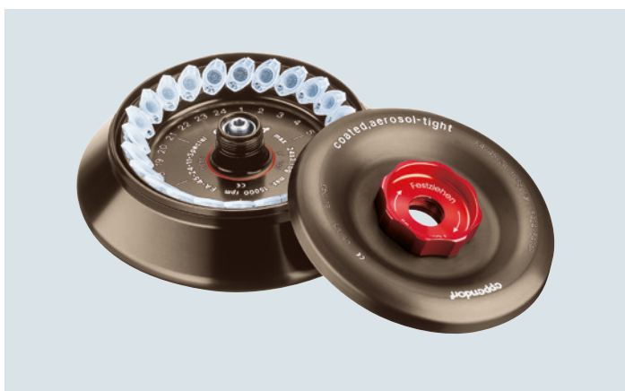
Aerosol-tight rotor for 24 × 1.5/2 mL tubes with PTFE-coating for high chemical resistance. Provides speed up to 21,130 × g /15,000 rpm (FA-45-24-11-Special; Order no. 5424 700.004).
