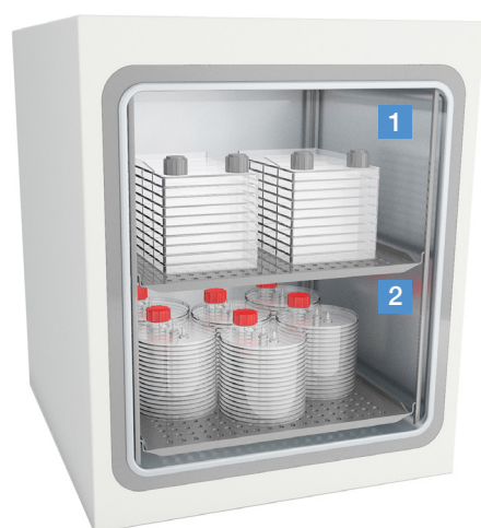
Fig. 1: Standard incubator, e.g. HeraCell 240 (Thermo Fisher Scientific) Incubator size internal dimensions: W 56 cm, H: 67 cm
