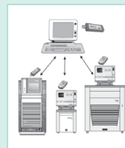
PC and Wireless USB Stick to control and monitor up to 8 JULABO instruments
